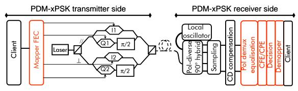
Figure 1: Example of a versatile PDM-xPSK transponder architecture. Left-hand side: transmitter, right-hand side: receiver. The red boxes indicate the parts of the transmitter and receiver sides that require a redesign compared to the legacy 100 Gb/s PDM-QPSK transponder architecture.
