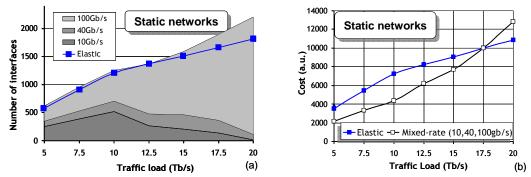
Figure 2: Number of interfaces required for the mixed-rate and elastic networks (a) and whole cost of the two network scenarios (b) as a function of the transported traffic load, static dimensioning is performed.
