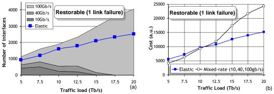
Figure 3: Number of interfaces required for the mixed-rate and elastic networks (a) and whole cost of the two network scenarios (b) as a function of the transported traffic load, the dimensioning is performed such as the network is resilient for one link failure.
