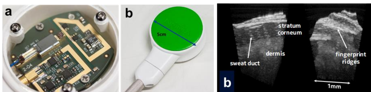
Figure 2. (a) OCT head. PCB board with mounted optical engine. (b) Two views of the in-vivo 3D rendered OCT data of approximately 1.3 \times 1.3 \times 1.5\text{mm}^3 region of a fingertip.
